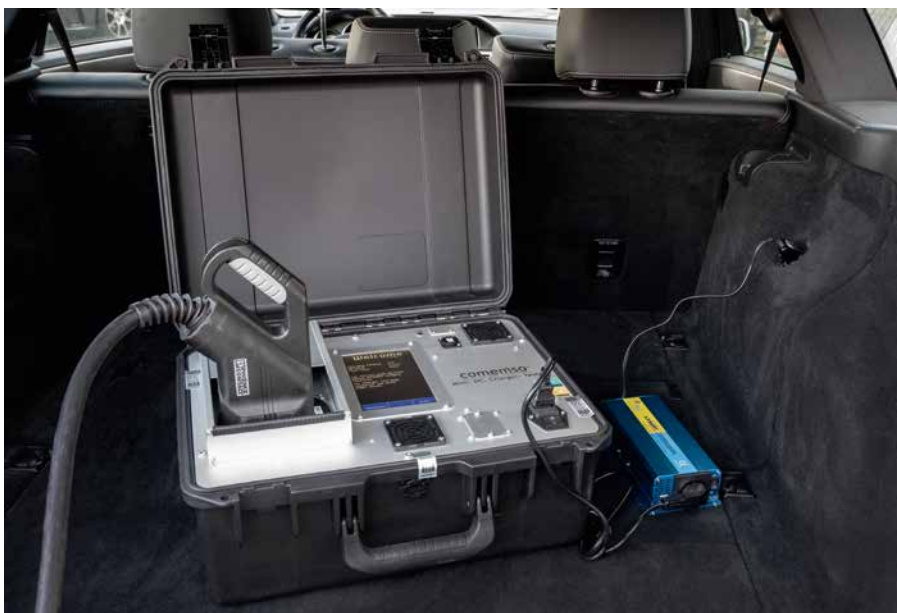
Field setup in the trunk with 12V car cigarette lighter, connected through a pure-sine wave 1kW power inverter. The inverter is not part of the comemso scope of delivery.
