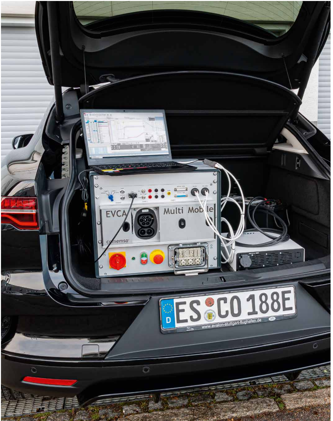
comemso EVCA Multi Mobile + Laptop, inverter (12V to 230V) and battery. (Additional components are not offered by comemso.)
